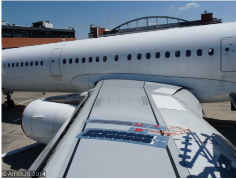
Figure 8: A321 left wing implementation of the wireless sensors together with the battery-free power supply based on solar energy harvesting and storage on supercapacitors.
