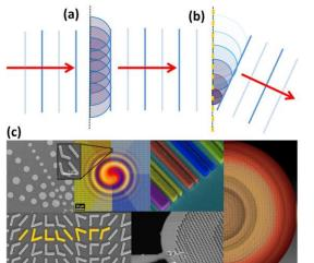
transmitting metasurfaces. (c) From left top to right bottom, multi-wavelength metasurface antenna [2], vortex plate[1], multi-wavelength achromatic lens [5], plasmonic V-shape metasurface[1], free standing flat lens.
