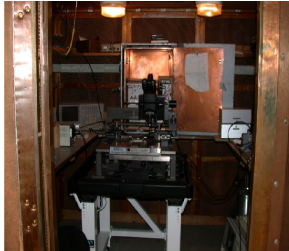
Faraday shielded room (LF noise)
