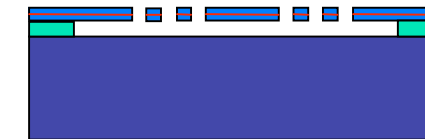
Membrane release (chemical etching)
