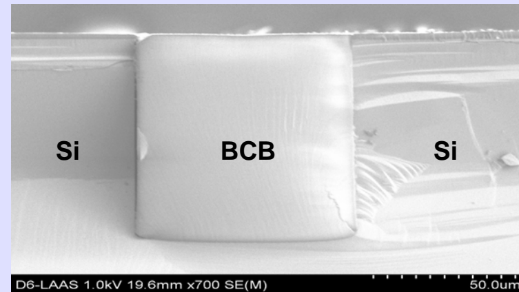
3. Central trenches and trench termination after CMP of the BCB at the surface
