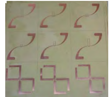
Antennas fabricated on 12"x12" in LCP Film
