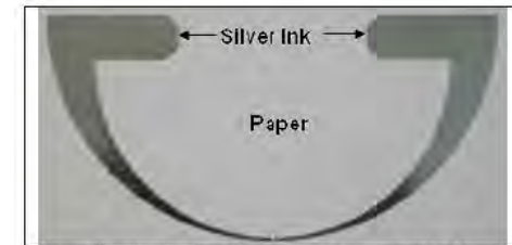
Figure 1. Silver based half-wavelength tapered-width U-shaped antenna Antenna on Paper
