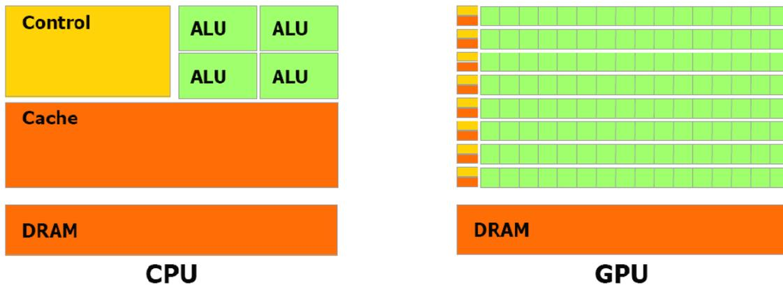
FIGURE IV.2 – Architecture CPU et architecture GPU (NVIDIA).
